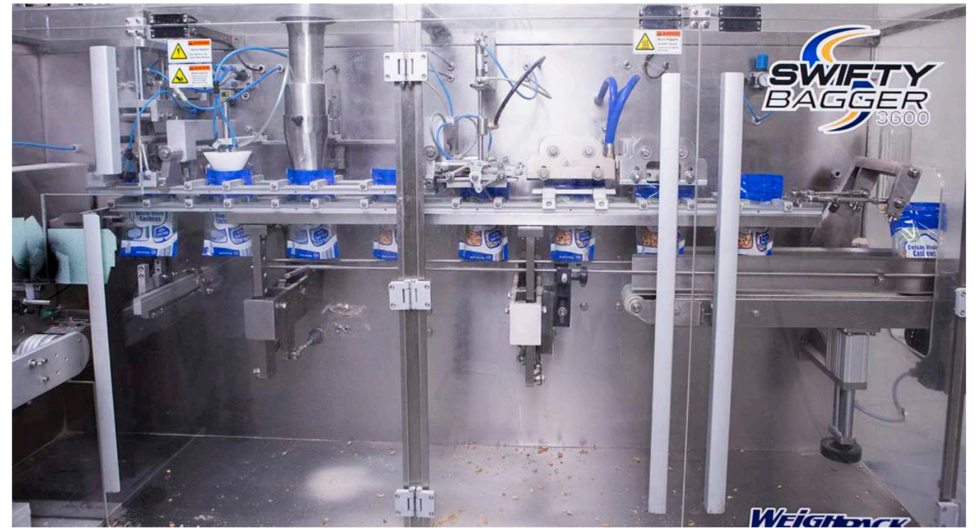
Installed at the Redland Foods facility earlier this year, the fully-automatic Swifty Bagger 3600 machine from WeighPack Systems forms the heart of the plants RSU (resealable stand-up) pouching line, producing an average of 40 stand-up pouches per minute in continuous operation that is designed to facilitate remarkably quick product changeovers.
