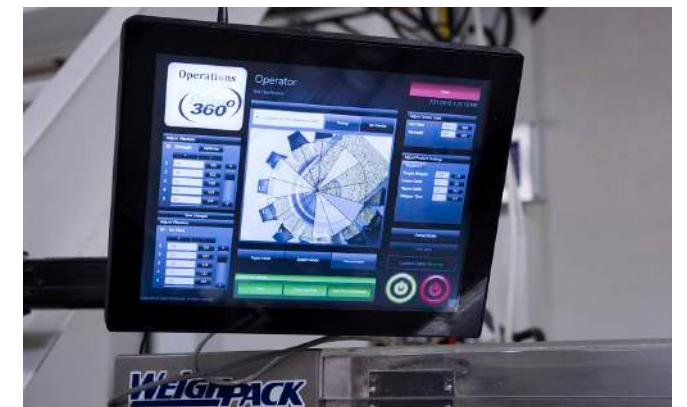
A video monitor on top of the Swifty Bagger 3600 provides machine operators with real-time camera footage and operating status for the PrimoCombi scales above.
