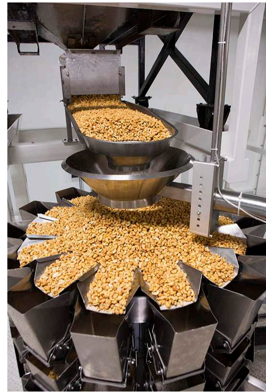
WeighPack supplied Redland plant with fully-automatic, 14-bucket PrimoCombi weigh scales for high-precision dispensing of bulk product into the Swifty Bagger
