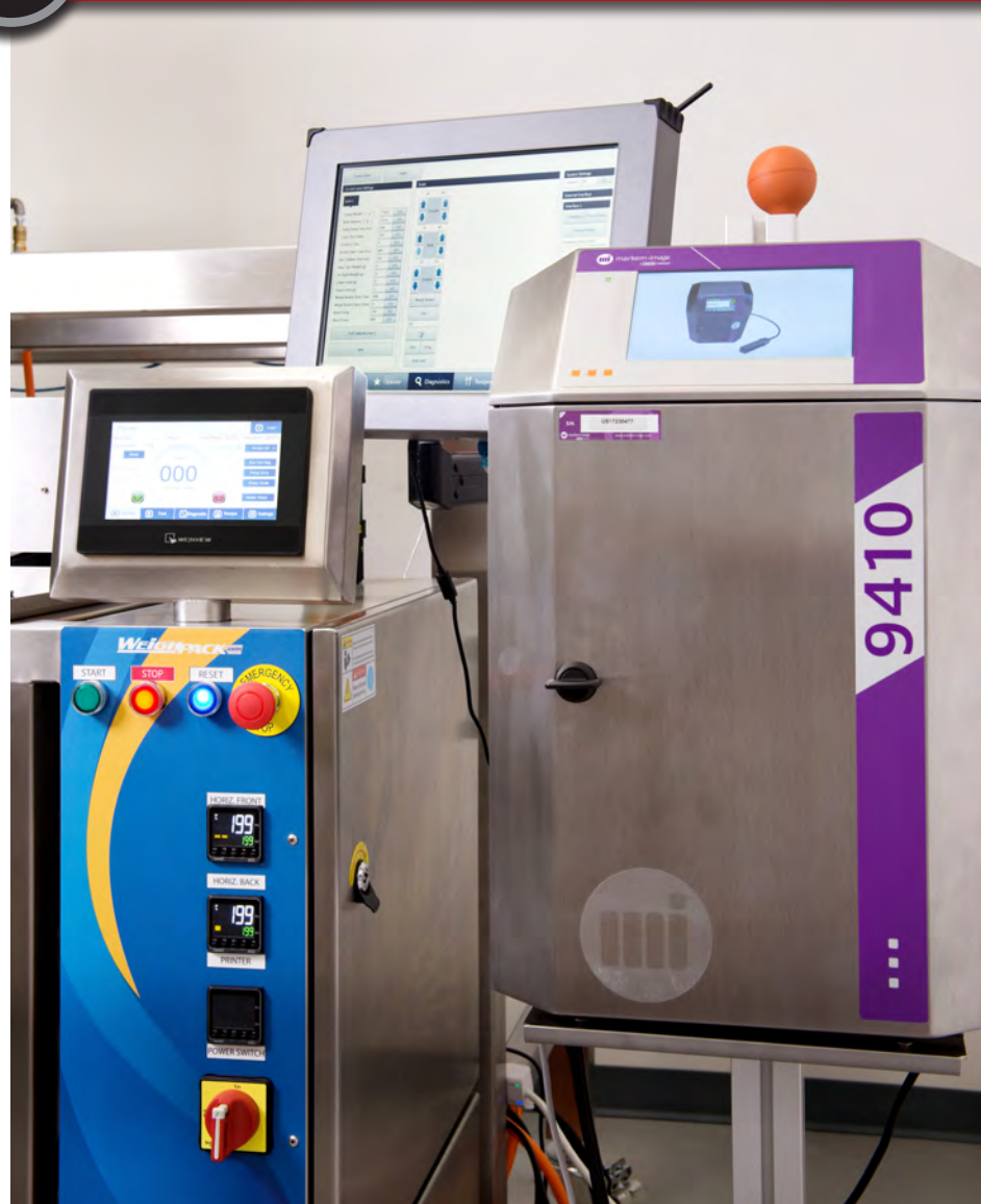
Wingreen utilizes a Markem-Imaje 9410 small-character for application of best-before dates onto the packs of dried blueberry and dried cranberry products.
