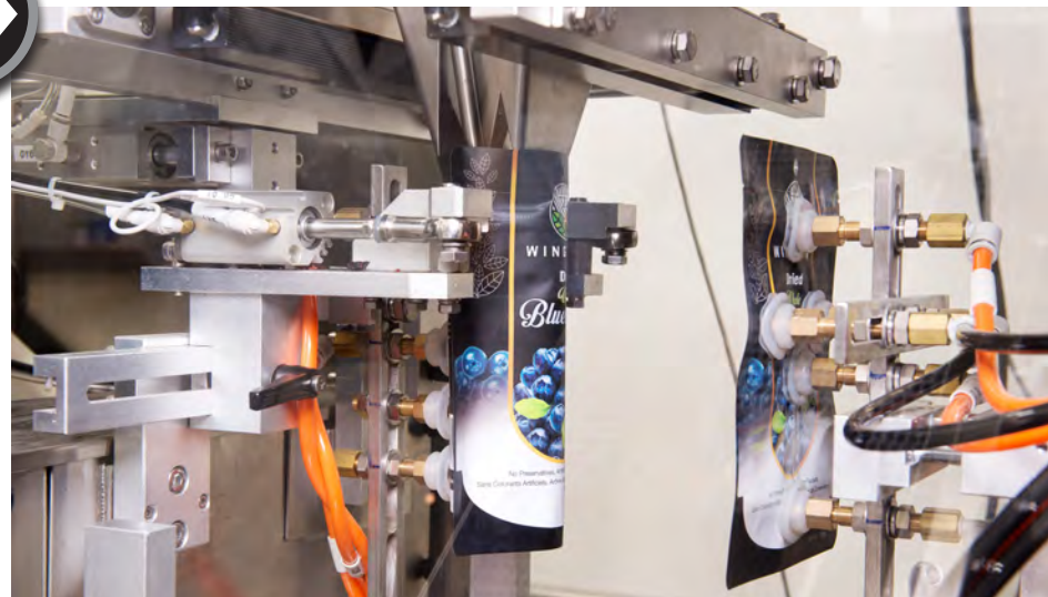
A close-up of the magazine holder on the WeighPack Systems’ Swifty Bagger Jr. bagging system gently pulling a stand-up resealable plastic pouch to the filling and sealing area of the machine at the 3,000-square-foot Wingreen berry packing facility.
