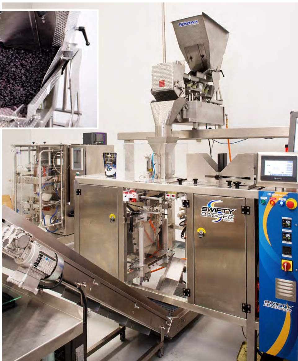
Purchased via Paxiom Group, the Swifty Bagger Jr. manufactured by WeighPack Systems is run by Wingreen at speeds up to 12 packs per minute, and not only helps the company provide packaging savings, but also forms packs that are eye-catching at the retail level.
