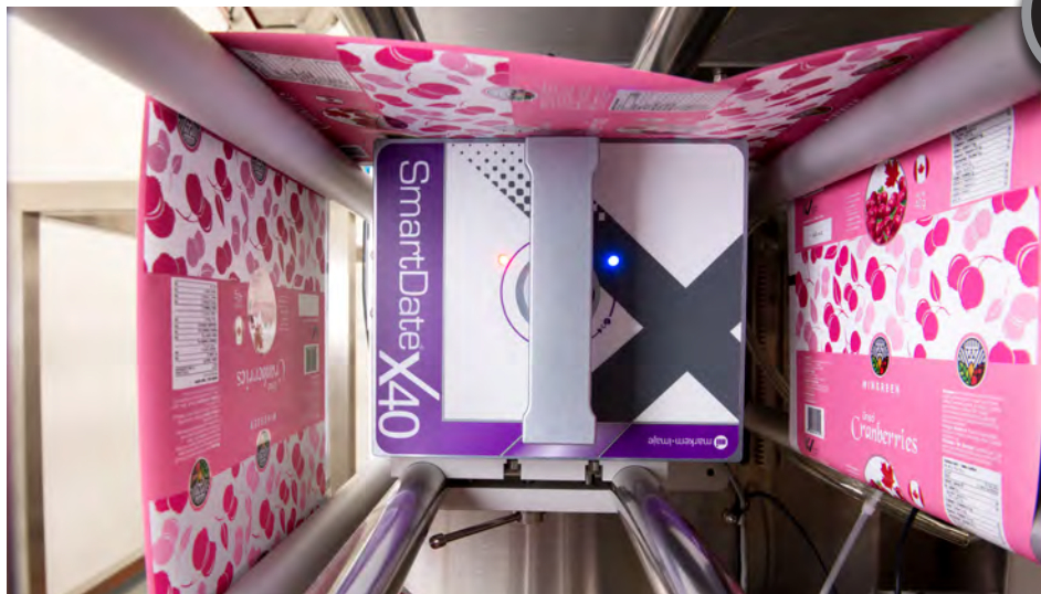
Within the VerTek 800 bagging system from WeighPack Systems, a Markem-Imaje SmartDate X40 thermal transfer printer adds lot-code and best-before data to flexible bags of Dried Cranberries on one of two production lines at Wingreen.
