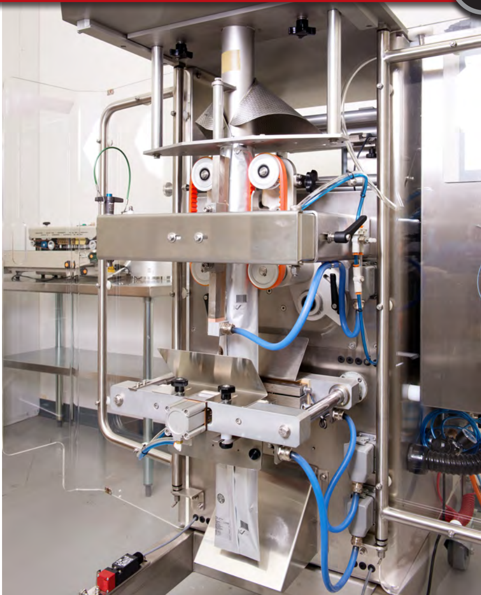
In early-2017, Wingreen purchased a VerTek 800 from WeighPack Systems to form-fill-seal smaller packs of dried berry products at speeds up to 16 units per minute.
