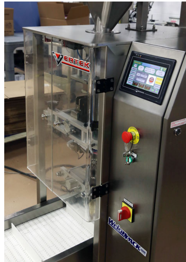
The WeighPack VerTek Junior bagger at Terra Cotta Food is placed off-center from the PrimoCombi weigher with an angled slide to ensure a gentle drop of cookie products.
