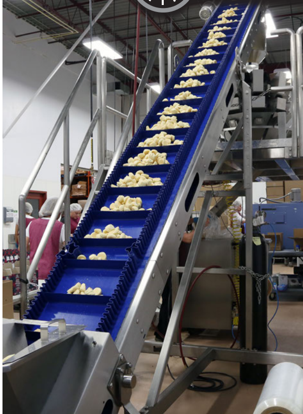
Part of the WeighPack Systems solution, shortbread cookies move up a stainless-steel, sanitary-designed vertical conveyor to deposit the baked goodness gently onto a Weigh-Pack PrimoCombi multihead weigher.
