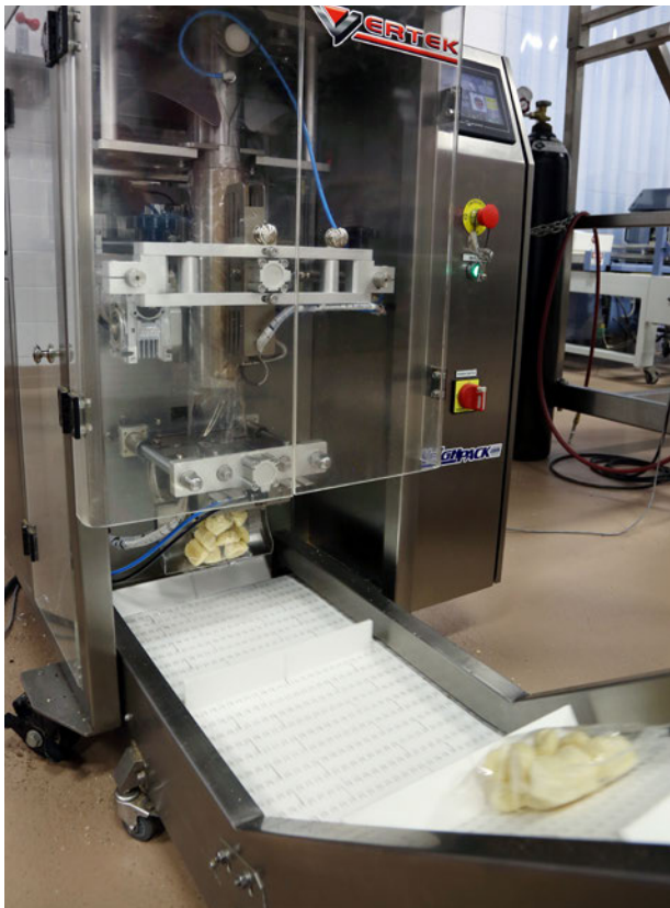
A VerTek Junior vertical form-fill-seal bagging system built by WeighPack Systems, a division of Paxiom Group, delicately packs bags of shortbread cookies at a rate of 45 packs per minute at Terra Cotta Food.
