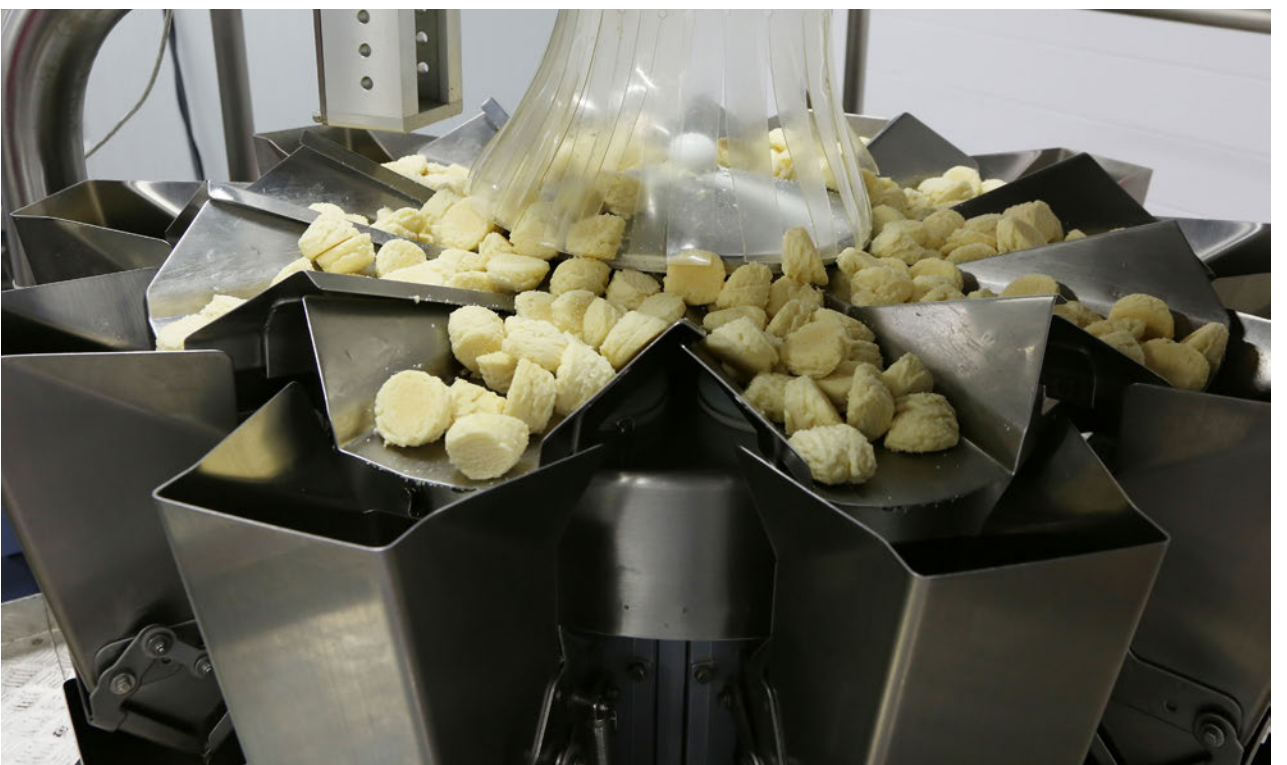
Because shortbread cookies crumble easily from over handling, the 10-head PrimoCombi automatic weighing system, designed and manufactured by WeighPack Systems, weighs product to within a single gram of tolerance before gently sliding it down a special-designed angled chute to create a softer landing spot for the cookies in the bagger below.
