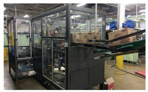
Prior to purchasing the case packing equipment, this beverage napkin line line used an employee to hand pack boxes and run them through a tape sealer. That labor has now been automated out of the line.
